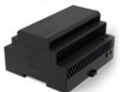
SL2873 Rev. 1 Switching Power Supply 24V dc 6.25 A DIN rail mounting Dim.: 6 modules 105x90x54.5 mm
