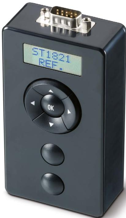
Configuration Control SC for production, assembling and test of blinds. The control of the blinds is operated via the data wire of the blind.
