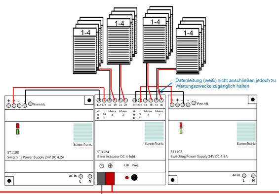
KNX bus line. Switches will be connected to this line. Software it will be determined which blinds need to respond to what switch
