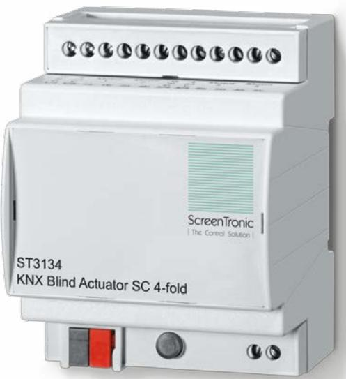
The KNX Blind Actuator is specially designed for the control of blinds in insulating glass or for applications with high demands on precise control. The Actuator is specific for the control of 24V SC brushless motors via a 3-pole wire. Every output is for connection of a single blind, which gets the power through 2 wires and is controlled very exactly with the 3rd wire (communication).
