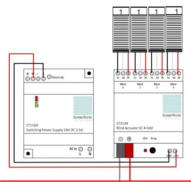
KNX bus line. Switches will be connected to this line. Software it will be determined which blinds need to respond to what switch
