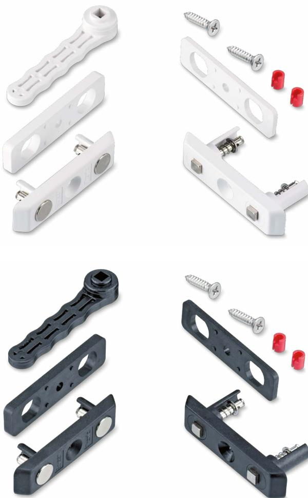
The tappet contacts ST9121 (white) and ST9122 (black) are suitable for transmission of electricity to windows or doors. A permanent electrical contact stability is ensured by a strong magnet that attracts the magnetic tappets. This contacts work entirely without access ramp, which allows the contacts to close from each position and side. As a result, the contacts are qualified for both normal window, turn/tilt doors as well as for lifting/sliding doors.
