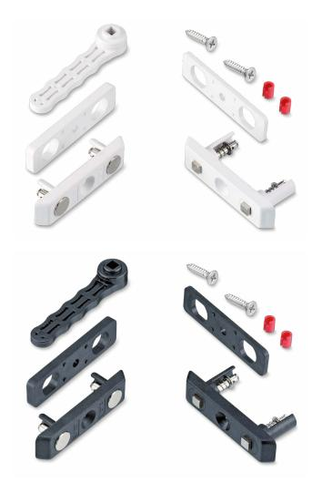
The tappet contacts ST9121 (white) and ST9122 (black) are suitable for transmission of electricity to windows or doors. A permanent electrical contact stability is ensured by a strong magnet that attracts the magnetic tappets. This contacts work entirely without access ramp, which allows the contacts to close from each position and side. As a result, the contacts are qualified for both normal window, turn/tilt doors as well as for lifting/sliding doors.
